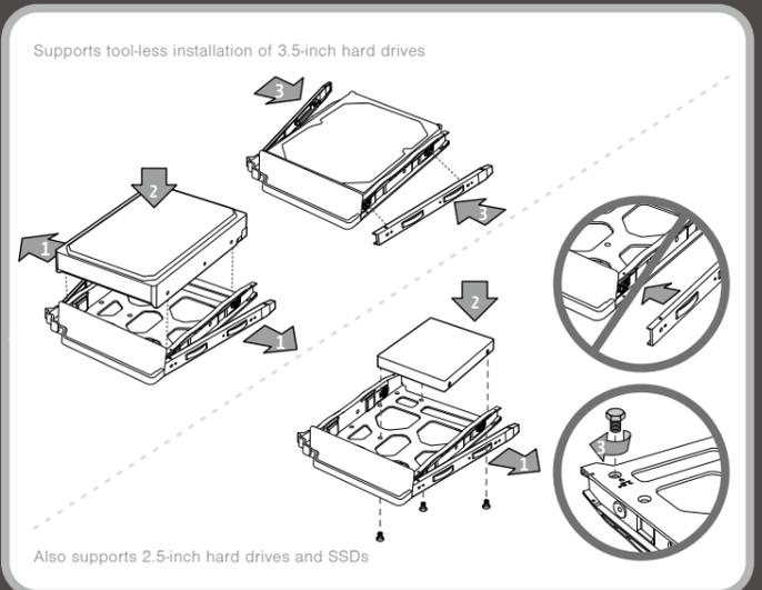
Supports tool-less installation of 3.5-inch hard drives
