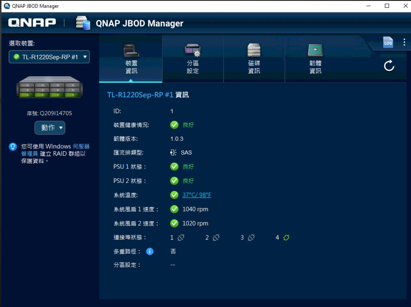
The screenshot displays the QNAP JBOD Manager web interface. The main content area shows the status for device TL-R1220Sep-RP #1. The interface includes a sidebar with a device selection dropdown and a main panel with tabs for Device Information, Partition Settings, Disk Information, and Firmware Information. The Device Information tab is active, showing a list of system metrics.
