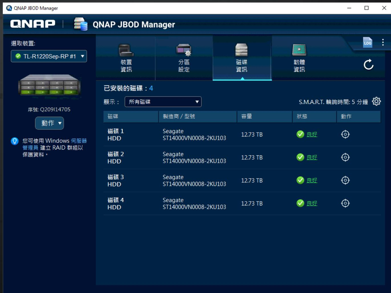
The screenshot shows the QNAP JBOD Manager web interface. On the left, the selected device is 'TL-R1220Sep-RP #1' with serial number 'Q209114705'. The main area displays '已安裝的磁碟 : 4' (4 installed disks). A table lists the disks with their manufacturer, model, capacity, status, and actions.
